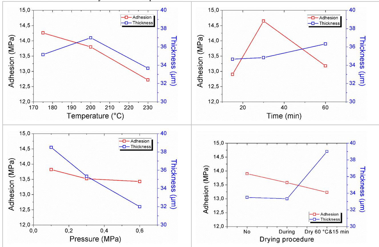
Fig. 4. Adhesion and joint thickness dependence on joining temperature, time, applied pressure and drying procedure
