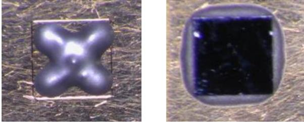
**Fig. 1.** Deposited paste (left) and chip placed into paste, chip size 3x3x0.52 mm
