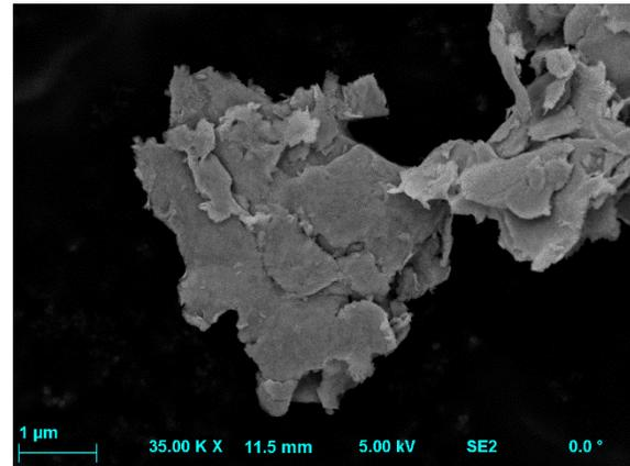
**Fig. 3.** SEM image of Ag particle – flake shape
