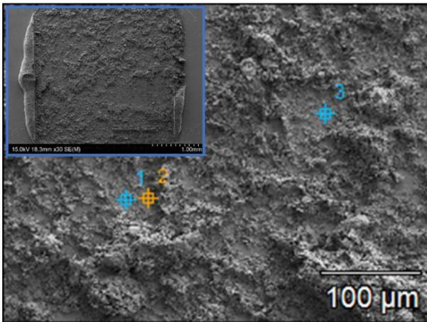
**Fig. 6.** SEM image of Cu substrate with NiAu metallization after chip removal, whole chip area shown in inset. EDS analysis in marked points:
